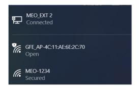
**4)** Once a connection has been established with the interfaces "AP" MAC address, open a Web Browser and enter the configuration page IP address
